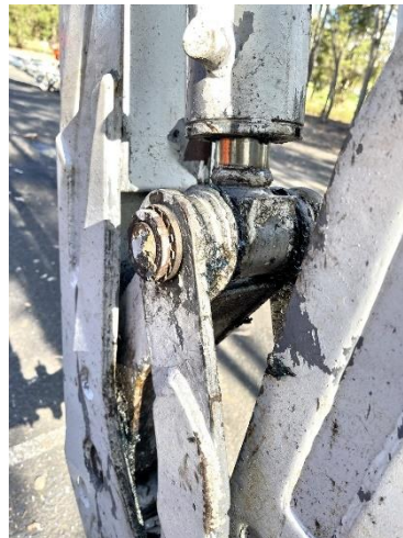
Fig 2. Worn bushes 3 rd to 4 th boom arm
